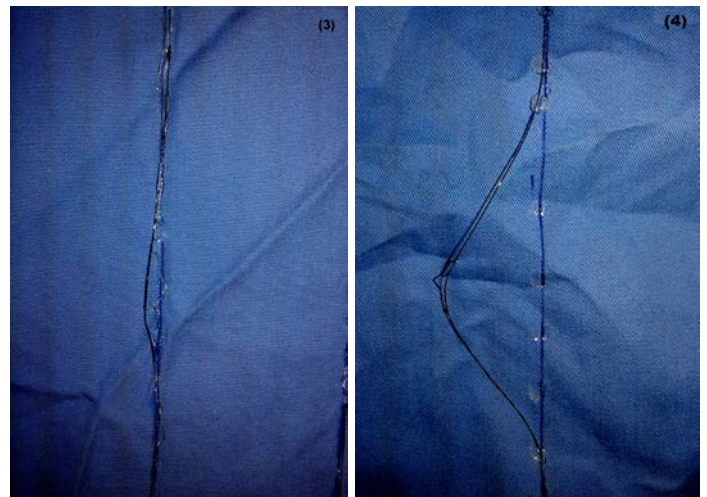
Fig. 8. Problems occurred after heat treatment and washing for sample; (3) on the left side, and (4) on the right side
