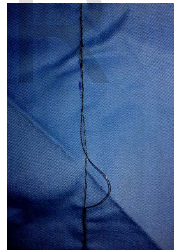
Fig. 9. SMA Wire tends to bend and slip among the stitches after washing
